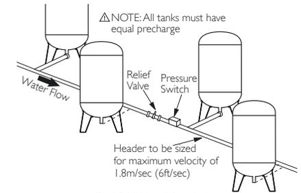
Fig. 1.5 Multi-tank Installation
